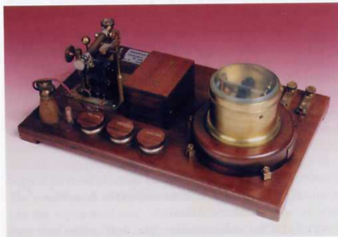
Fig 4. A reconstruction of the Siemens and Halske receiver supplied to the Boers (Siemens AG)
